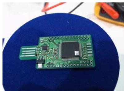
Embedded electronics for semi-autonomous robot
